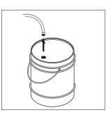
**STEP 1:** If using an optional detergent injector, place the detergent line in a bucket of water allowing detergent to be flushed from system.
